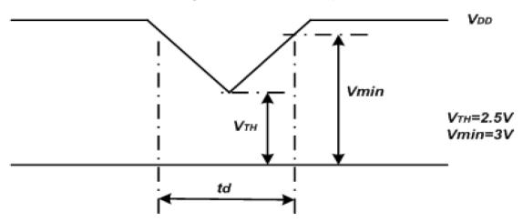
If  $V_{TH} < V_{DD} \le V min$ , then  $t_d \le 10 ms$ ; When the voltage return to normal our panel must revive automatically.
